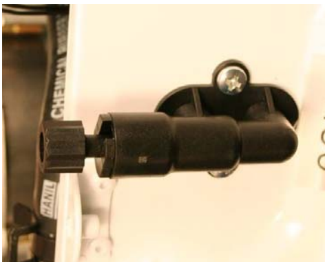
Manual Auto Fill Valve located on base of cabinet
